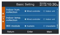
In basic setting interface, press Up/Down key to adjust unit number; press Left/Right key to move the cursor. Some functions are reserved for some models and the information is gray.
